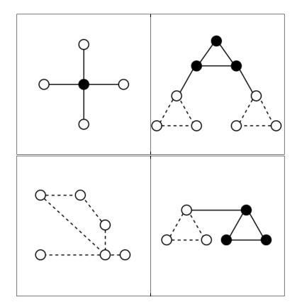
Figure 1: Possible network topologies. Black nodes are servers, white nodes are mobile devices. Filled edges represent Internet connections, while dashed edges are Bluetooth connections.
