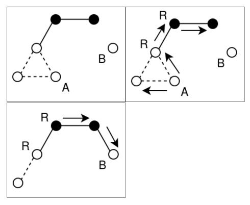
Figure 4: A is sending a message to B. The message is buffered on relays (marked R), and delivered when B connects.
