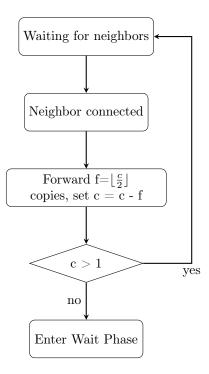
Figure 5: Flowchart of a node in the spray phase for a given message.
