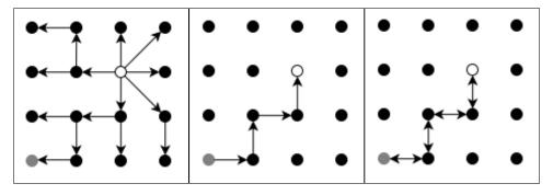
Figure 7: Visualization of the AODVv2 route discovery process.
