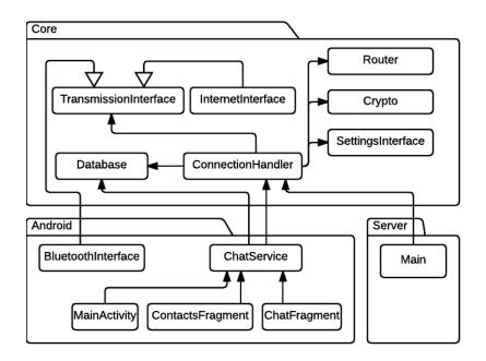
Figure 3: Class diagram of the core, library and Android projects. Only the most important classes are shown in this diagram.
