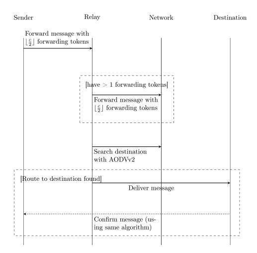
Figure 6: Message transmission between devices. Note that the sender performs the same discovery actions as the relay. Additional relays are not shown.
